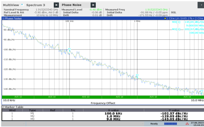
Figure 14 Phase Noise of the Integrated Oscillator at Divider Output (1.915 GHz)
